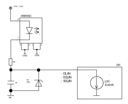
Figure 8: Circuit diagram for transmit LED HFBR-1505C
