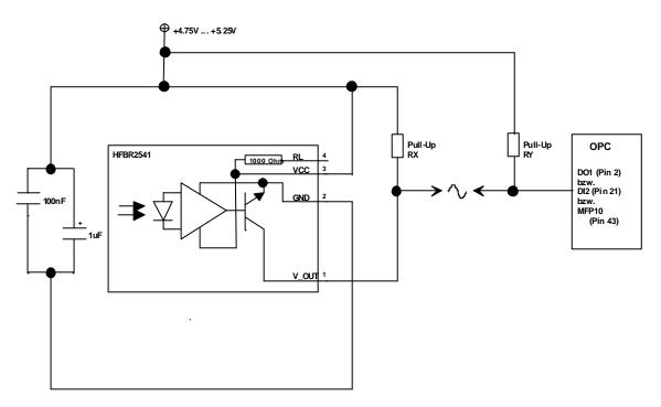
Figure 12: Circuit diagram for receiver HFBR-2541
