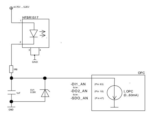
The Zener diode is an EMI protection measure (burst, surge). The resistor and the capacitor reduce the edge steepness of the very quick transmitter and also attenuate current noise from the SUPI 3 OPC. In terms of layout, all three components should be located as close as possible to the input on the protocol chip.
