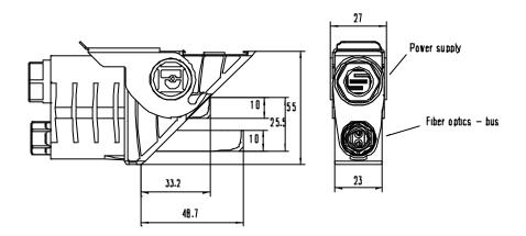
Figure 7: Rugged Line IP67 fiber optic hybrid connector
